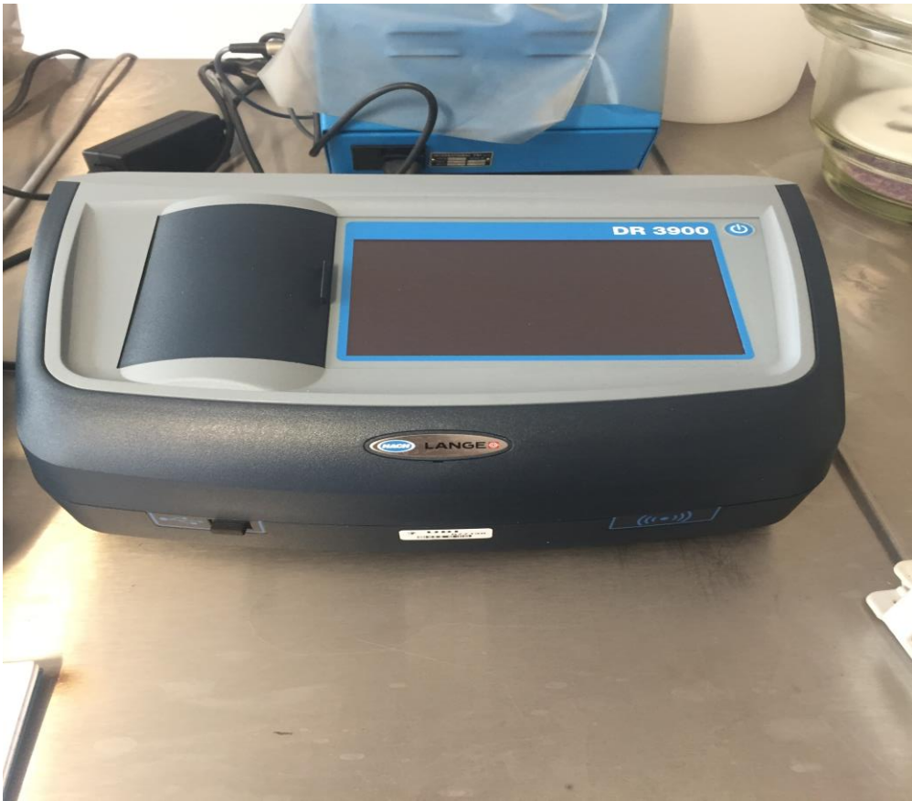
Fig. 3.6 - Spectrophotometer used for the analysis of the N and P assimilation.
