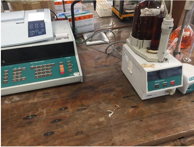
Fig. 3.4 - Titrator used for titulation of the samples for COD measurement
