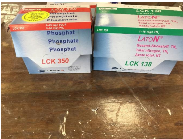
Fig. 3.5 – The kits used to analyse the Nitrogen and Phosphorous concentrations
