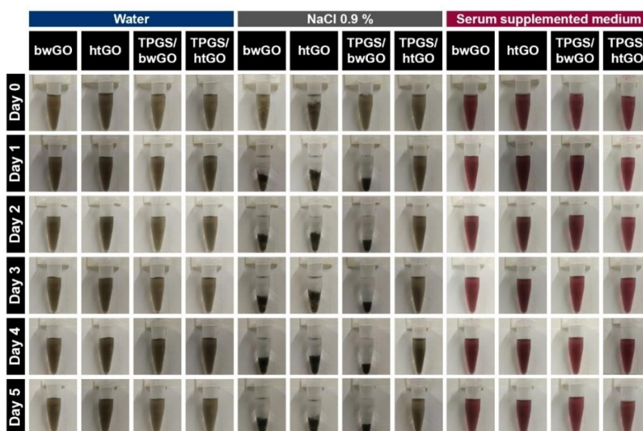
Figure 4.4. Macroscopic images of bwGO, htGO, TPGS/bwGO, and TPGS/htGO in water, NaCl 0.9 % and serum supplemented medium (DMEM-F12 supplemented with FBS (10 %, (v/v))) taken over the course of 5 days (end-point of the study). bwGO and htGO promptly precipitated in NaCl 0.9 %. TPGS/bwGO precipitated in NaCl 0.9 % after an incubation period of 12 h.
