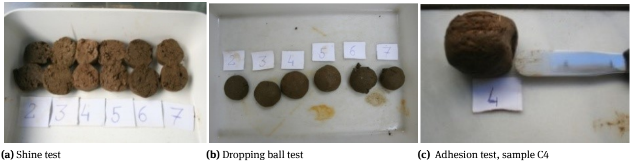
Figure 7: Shine, dropping ball, adhesion and water retention tests.
