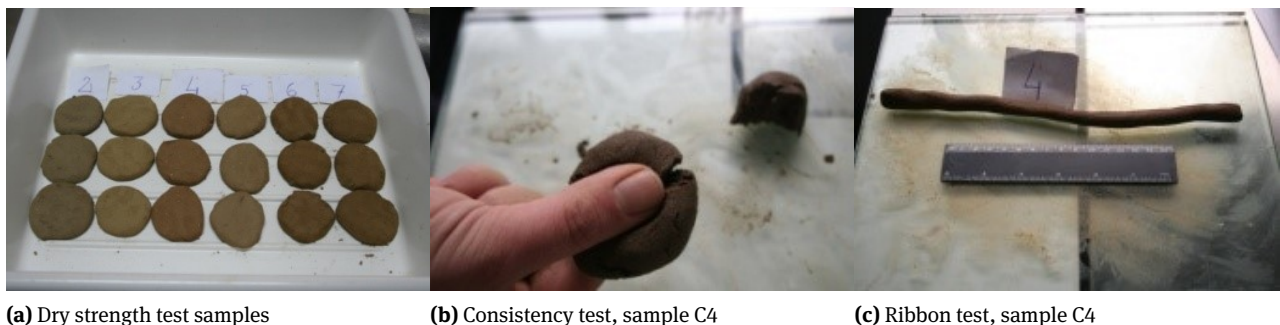
Figure 8: Dry strength, consistency and ribbon test.
