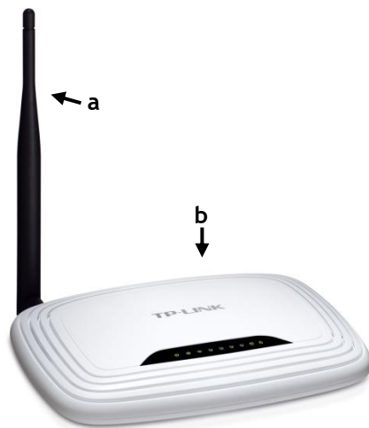
Figure 10: The internet router TP-LINK model number TL-WR740. A 150Mbps wireless router with 9V power and a frequency band of 2.4 GHz. a- Wi-Fi horn used to transmit and receive signals; b- Wi-Fi hardware. Adapted from 79
