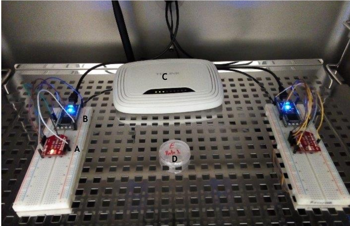
Figure 11: Disposition of the petri dish containing sperm cells for the exposure to the Wi-Fi network. A- Wifly; B- mbed; C- Wi-Fi router; D- The petri dishes are placed between the receptor and sender.
