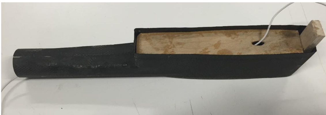
Figure 4.12 - Empennage support complete.
