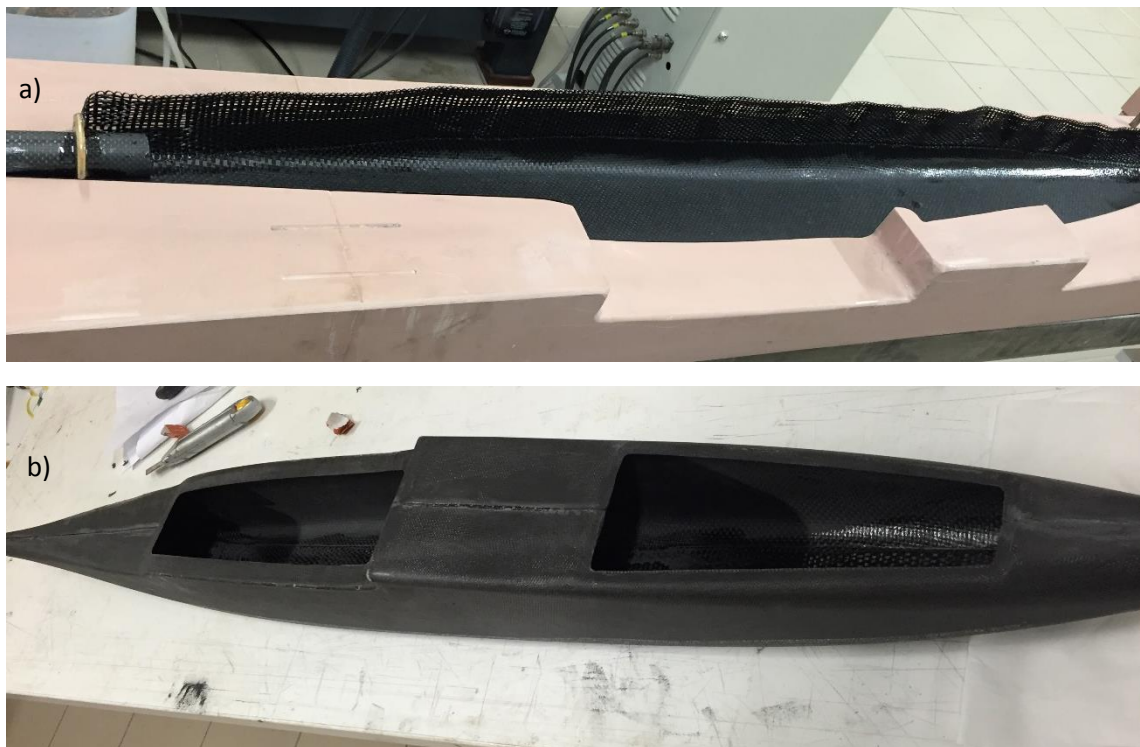
Figure 4.10 - Fuselage before (a) and after (b) be joined.
