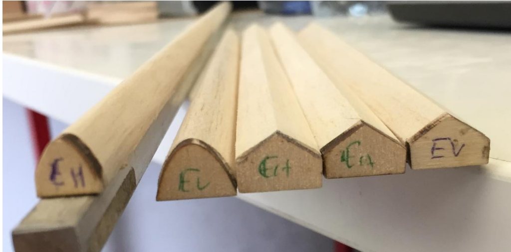
Figure 4.14 - Horizontal and vertical tail leading edges.
