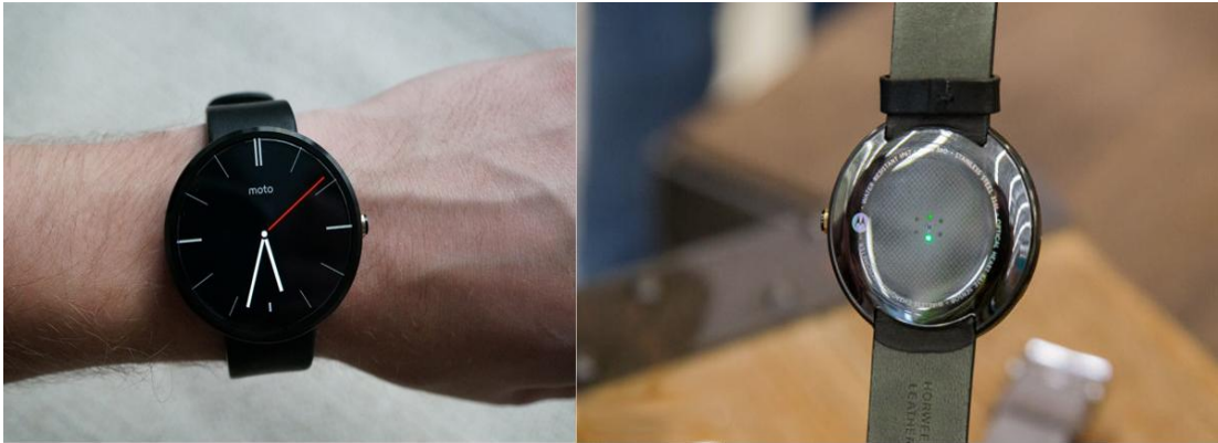
Fig. 31 - Moto 360 smartwatch front (left) and Moto 360 smartwatch back with optical heart rate sensor enabled (right).
