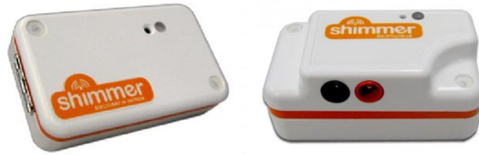
Fig. 32 - Example of two Shimmer modules: without any expansion board (left) and with a GSR expansion board connected (right).
