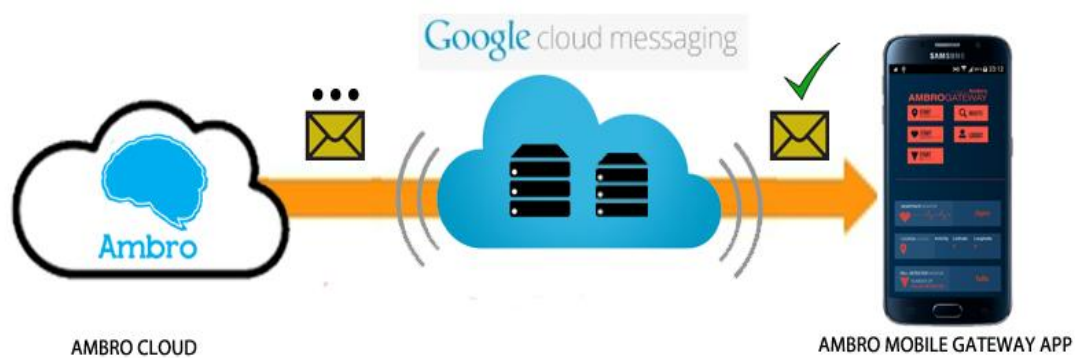
Fig. 43 - Illustration of the push notifications mechanism on the AMBRO system.
