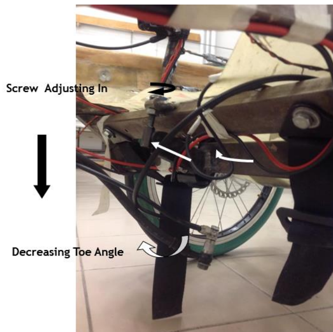
Figure 3.5 - Representation of toe angle tuning mechanism.
