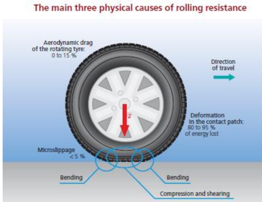
Figure 2.2 - Physical causes of rolling friction, [6].
