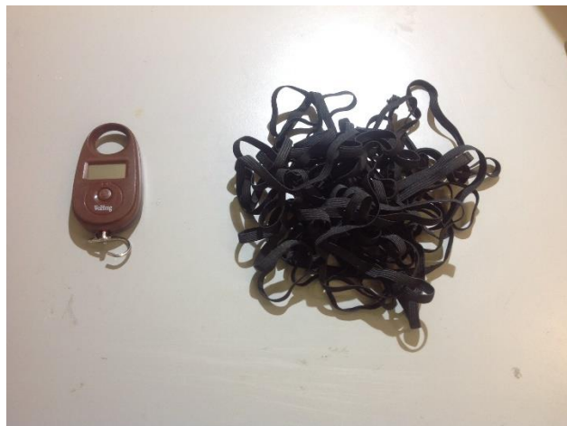
Figure 3.10- Dynamometer and elastic rubber band used in the rolling friction force measurements test.
