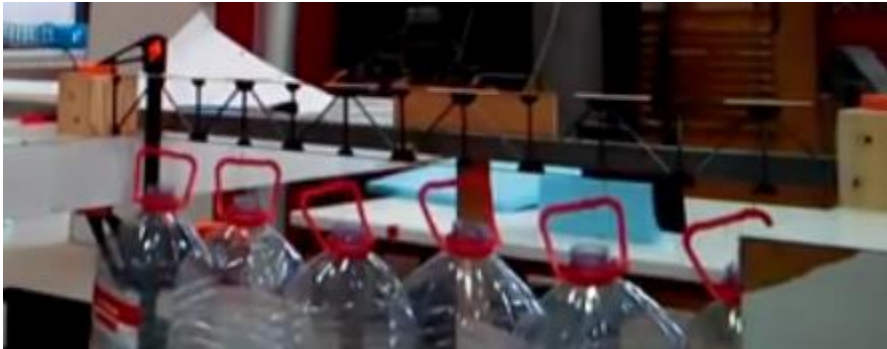
Figure 21: Experimental test applying 6 loads in the truss.
