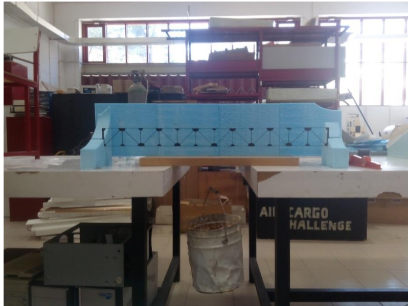
Figure 20: Experimental test applying one load in the center of the truss.
