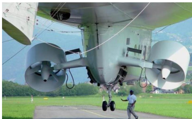
Figure 6. Vector Thrust Model (Prentice and Hochstetler, 2012)
