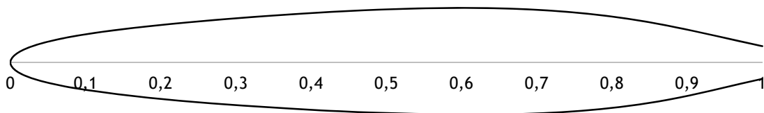
Figure 3.8 - Airfoil created on XFLR5 for the vehicle design
