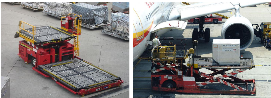
Figure 2. ULD loader composed by two platforms which can be raised and lowered independently [14].
