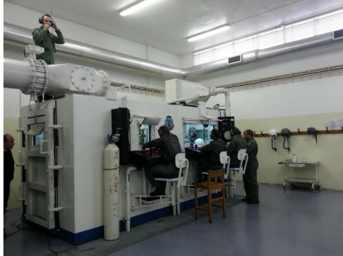
Figure 11: Hypobaric Chamber of Centro de Medicina Aeronáutica of the Portuguese Air Force.
