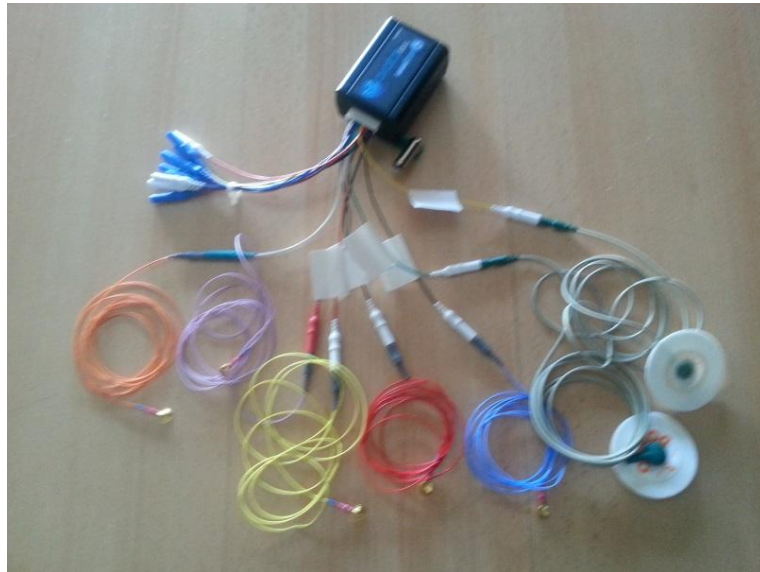
Figure 9: Avatar EEG equipment configuration.
