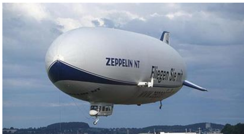
Figure 7 - Hélium Envelope and Vertical Thrust Provided by Vectoring Engines, ( http://brickmuppet.mee.nu/futurism/archive/2007/11 ).
