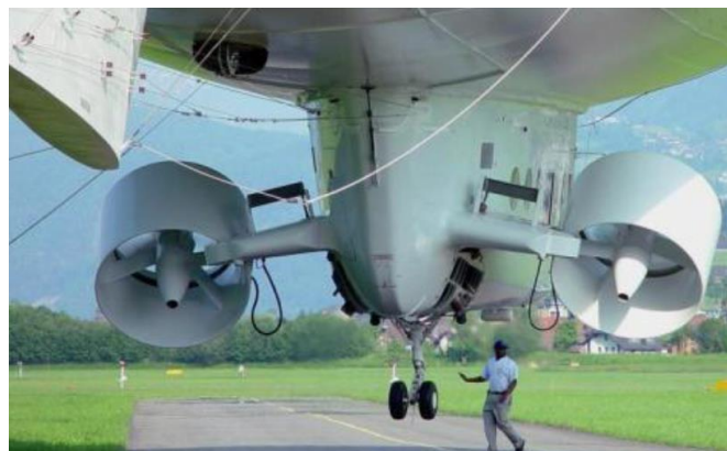
Figure 6. Vector Thrust Model (Prentice and Hochstetler, 2012)
