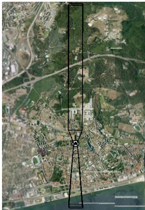
Figure 41 - Airship Surface-level and Obstacle Limitations Surfaces, Top View, (SketchUp)
