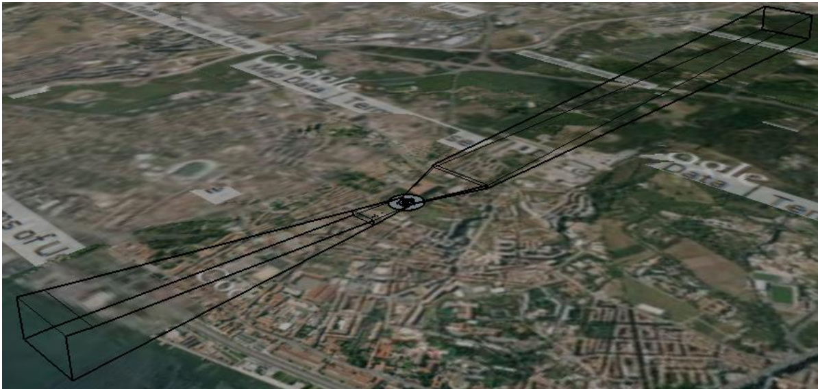
Figure 42 - Airship Surface-level and Obstacle Limitations Surfaces, Isometric View, (SketchUp).
