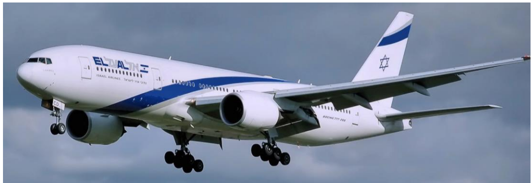
Figure 11: El Al Boeing 777-200ER, with RR Trent 895-17 engines [31].
