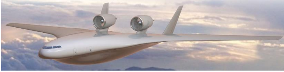
Figure 8: Future aircraft - engines above the fuselage in tail mounted pods [28].
