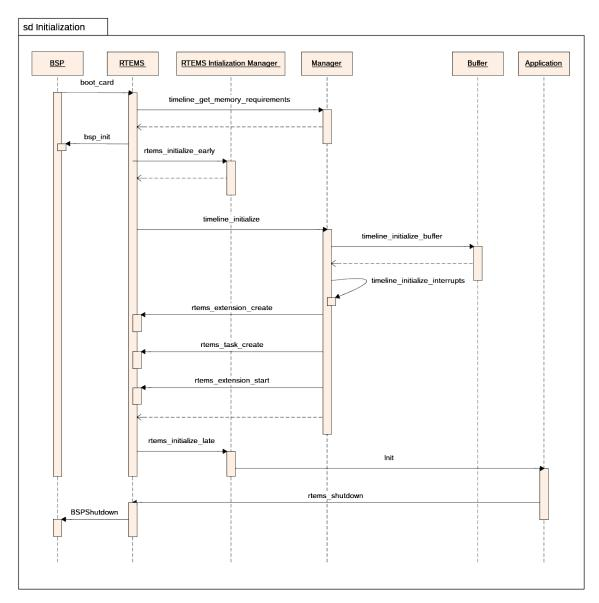
Figure 4.4: Monitoring Tool Initialization Sequence Diagram.
