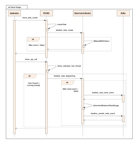
Figure 4.9: Monitoring Tool Stack Usage Logging Sequence Diagram.
