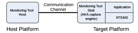
Figure 3.1: Monitoring Tool Platform.
