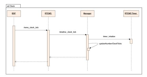
Figure 4.11: Monitoring Tool Clock Update Sequence Diagram.
