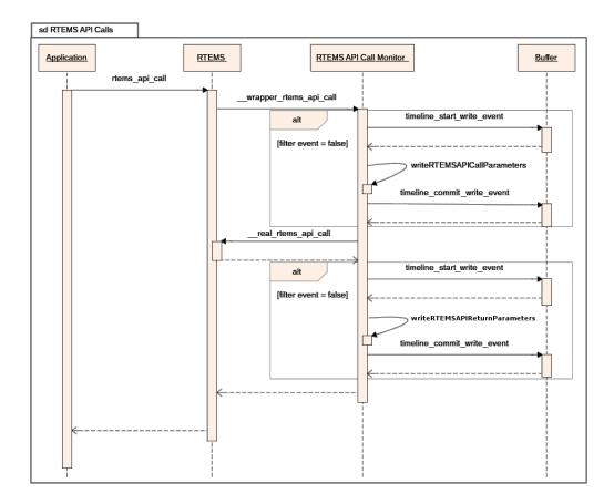
Figure 4.8: Monitoring Tool RTEMS API Call Logging Sequence Diagram.
