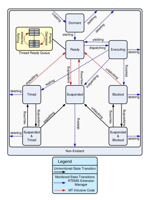
Figure 4.6: Monitored RTEMS Task State Transitions.
