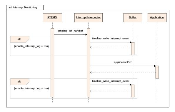
Figure 4.5: Monitoring Tool Interrupt Logging Sequence Diagram.
