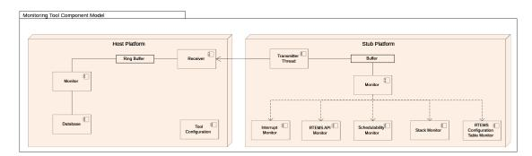
Figure 4.1: Relationship between the Monitoring Tool Major Components.
