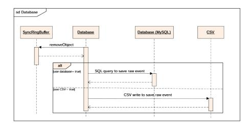
Figure 4.13: Monitoring Tool Database Sequence Diagram.
