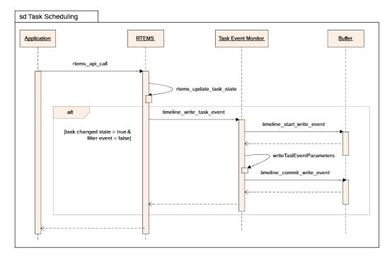
Figure 4.7: Monitoring Tool Task Scheduling Logging Sequence Diagram.
