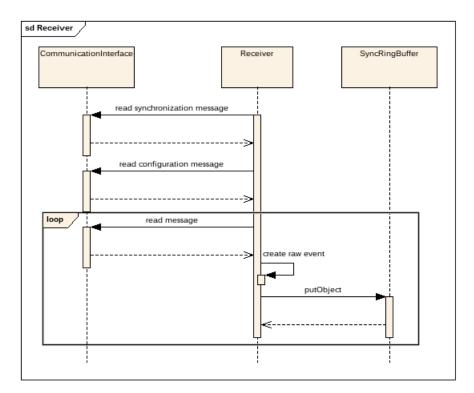
Figure 4.12: Monitoring Tool Receiver Sequence Diagram.
