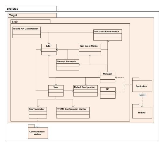
Figure 4.2: Monitoring Tool Stub Class Diagram.
