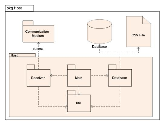
Figure 4.3: Monitoring Tool Host Class Diagram.
