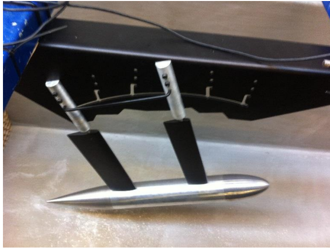
Figure A.1 - Full Prototype Configuration after manufacturing; Here, it can be seen the hull body at 20° of AoA during testing stages.
