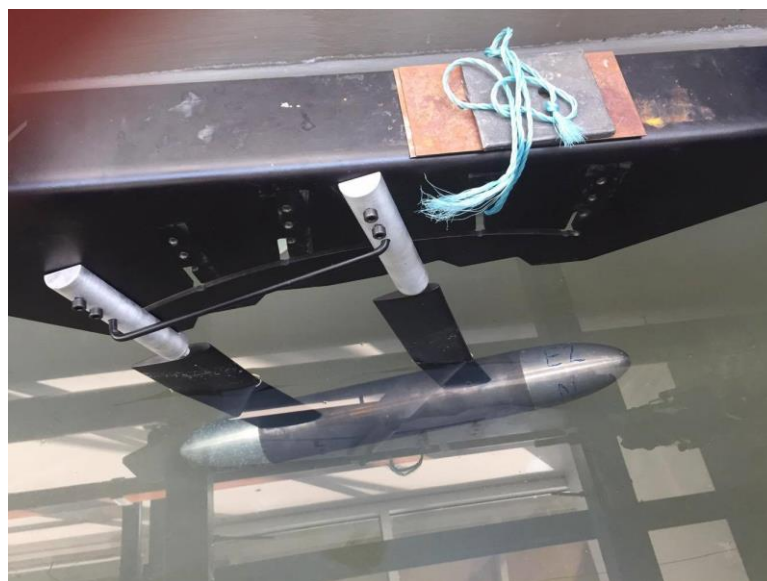
Figure E.2 - Towing Carriage with Weights; Here, it can be seen that depending on hull's AoA, the Weights position changes.
