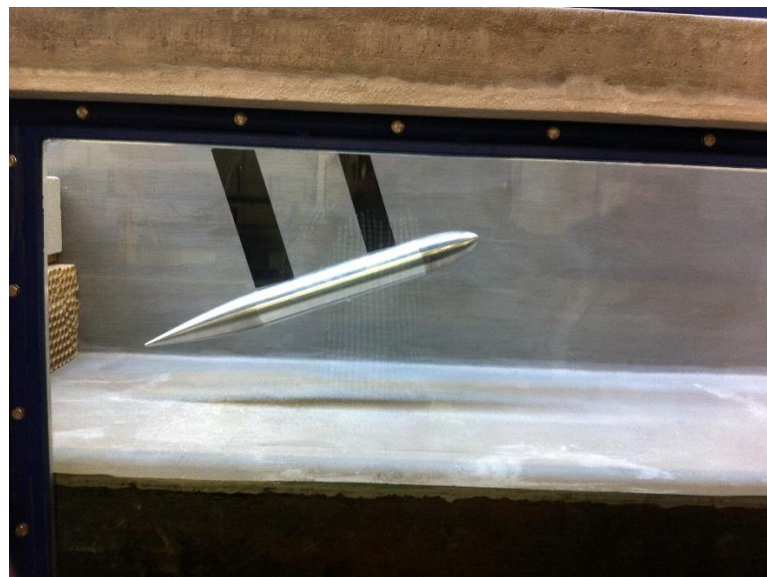
Figure B.2 - Model's attitude travelling at 20^\circ ; Here, it can be seen the hull body at the starting position.
