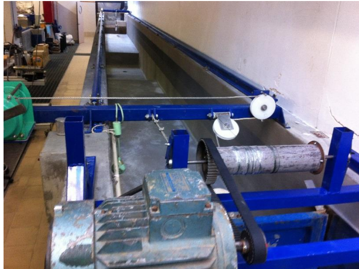
Figure B.1 - Towing tank without water; Here, it can be also seen a first unsuccessful mount configuration with a different motor.
