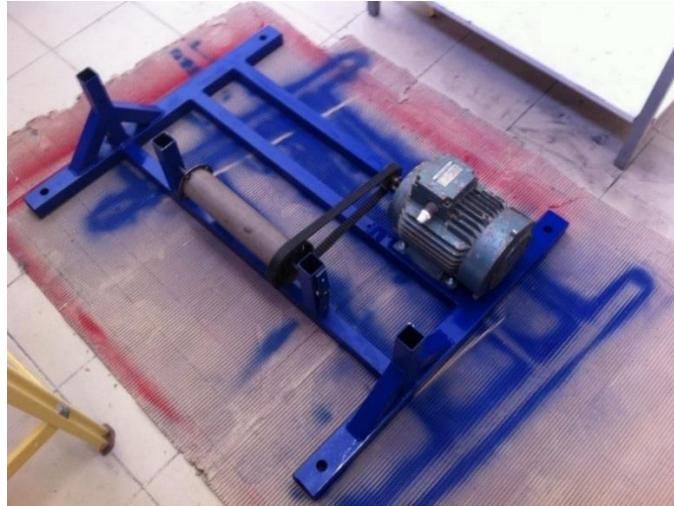
Figure 4.8 - Final metallic structure assembled before mounting at the towing tank.
