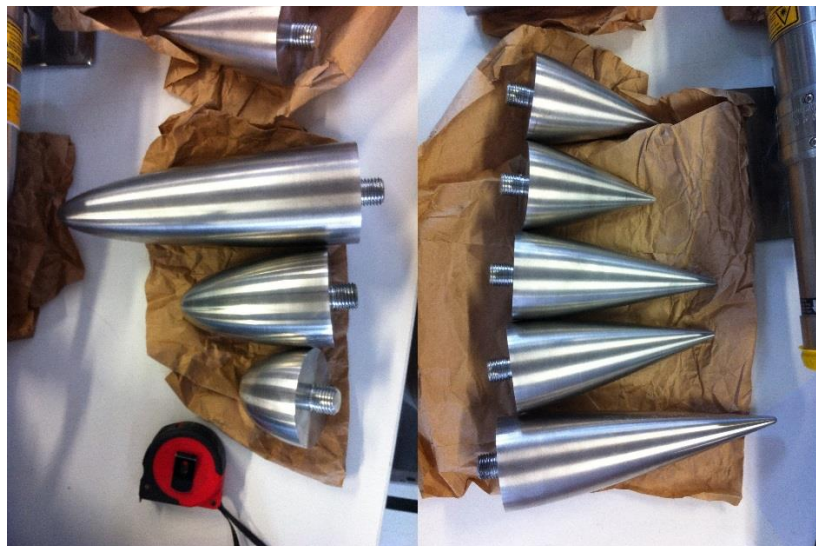
Figure A.2 - Nose and Tail configurations; Here, it can be seen several Nose/Tail configurations used on Experimental Tests.
