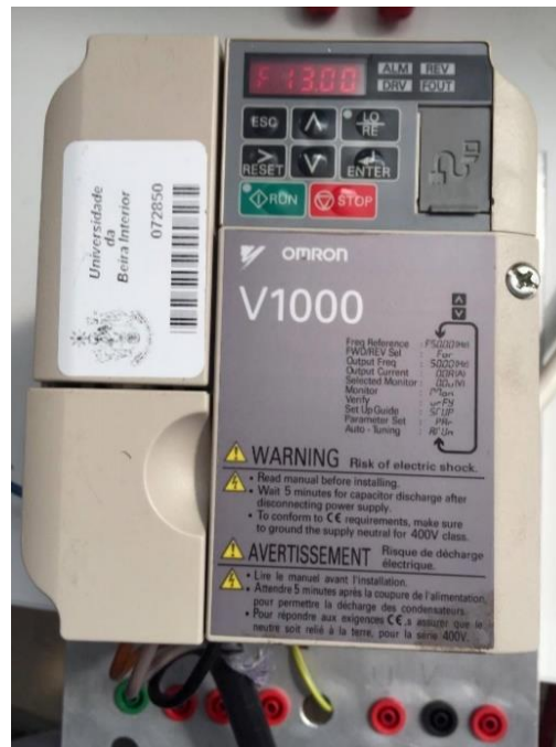
Figure D.1 - Frequency Inverter used; Here, it can be seen a pre-programmed run for 13 Hz (0.75 m/s).
