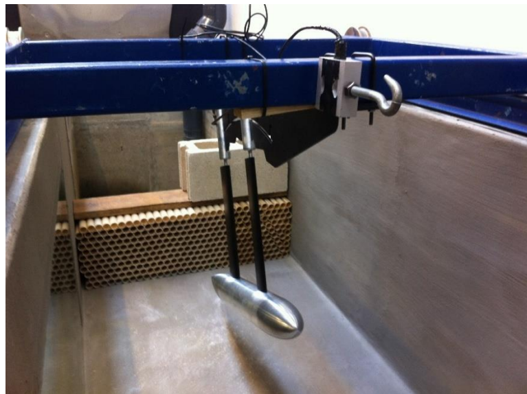
Figure C.2 - Initial Dynamometer used; Here, it can be also seen the tubes where the water entered on the Towing Tank.
