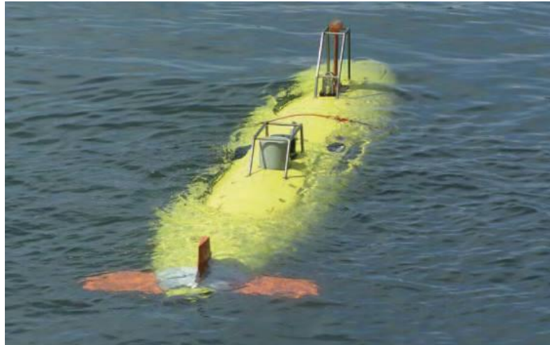
Figure 2.3 - REMUS 6000 operating near free surface (adapted from [22]).
