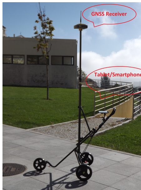
Figure 1.2: Device developed to acquire the GNSS and attitude observations
