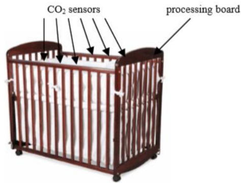
Figure 15 - Illustration of a crib with CO 2 sensors deployed around the baby. The sensors are connected to a processing circuit board.
