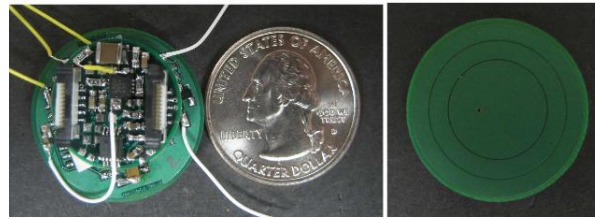
Figure 5 - Sensor for measuring heart rate without the need to put in suction contact with the skin.
