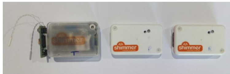
Figure 25 - Illustration of body sensors used on the proposed solution: a) temperature sensor; b) position sensor and c) respiration sensor.
