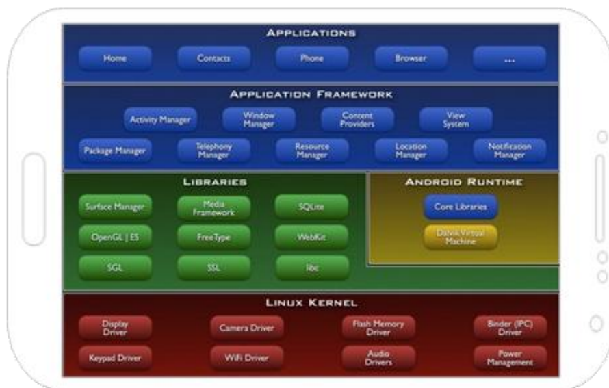
Figure 23 - Illustration of the Android OS architecture.
