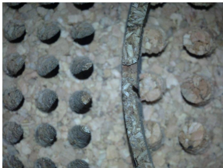
Figure 29 - Small tab that prevents any movement by the cork sample
