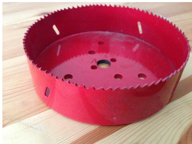
Figure 20 - Bi-metal 152 mm hole saw
