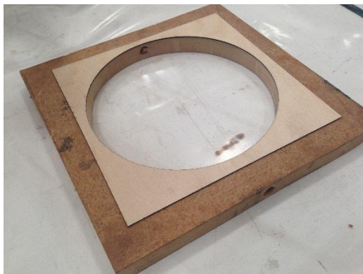
Figure 38 - New molds with holes (open)
