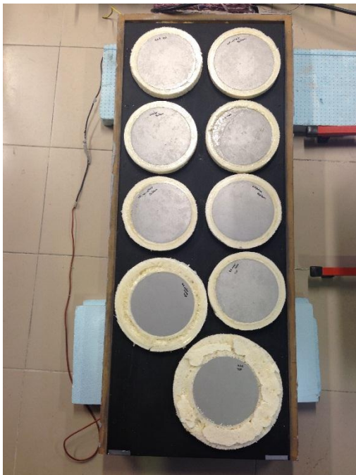
Figure 43 - Test samples placed on heating plate
