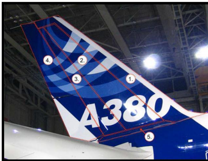
Figure 11 - VTP major structural assemblies (example A380). (Herrmann, 2005)
