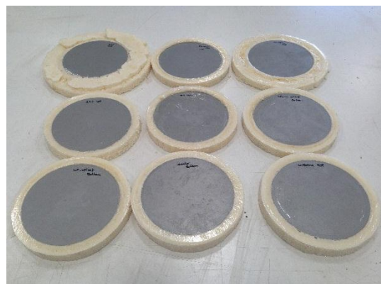
Figure 42 - Finished laterally insulated test samples
