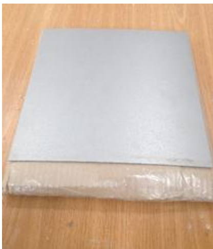
Figure 19 - Aalco 5754 square aluminum face sheets
