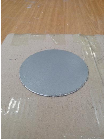
Figure 23 - Extracted Aluminum face sheet
