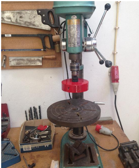
Figure 21 - Milling machine with hole saw
