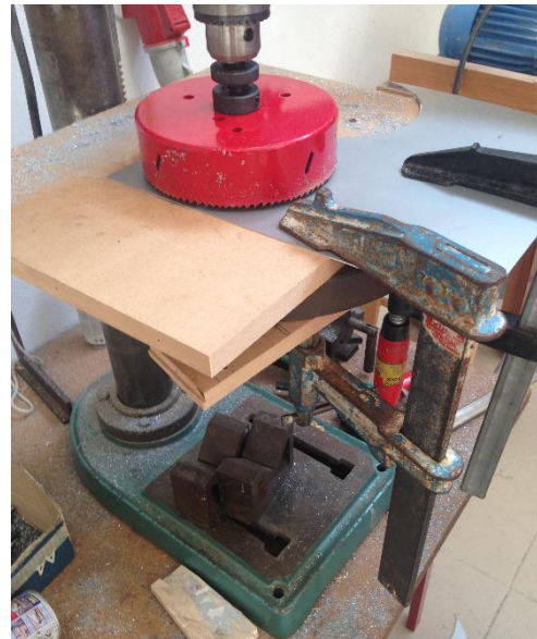
Figure 22 - Cutting process of the aluminum sheet
