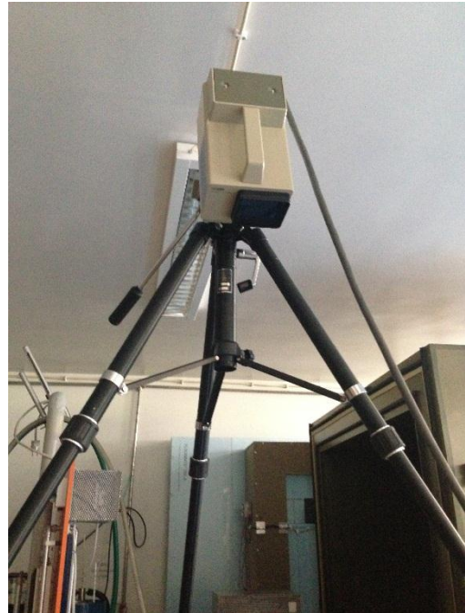
Figure 46 - Thermographic camera placed directly above the test samples
