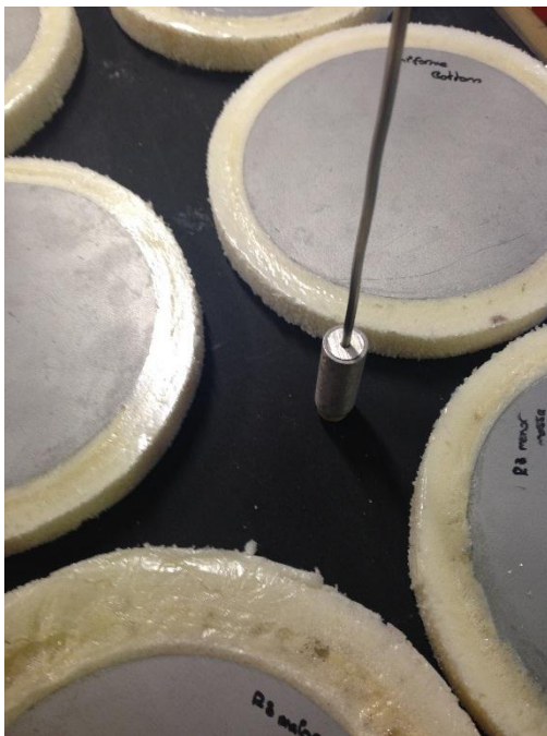
Figure 64 - Temperature measurement of the heating plate
