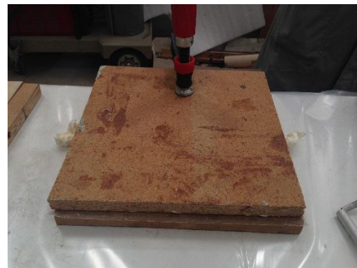
Figure 39 - New mold with cover and clamps (closed)
