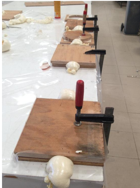
Figure 40 - Closed molds with fully expanded foam
