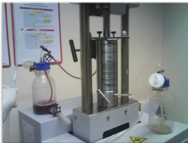
Figure 2.1 – French-Press equipment in use with fast-flow anaerobic kit assembled
