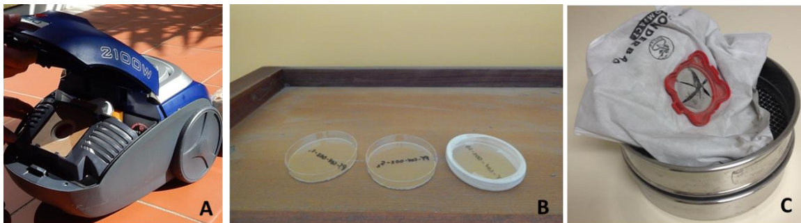
Figure 1. House dust sampling. (A) Household vacuum cleaner used for active sampling; (B) Petri dishes placed on the top of a shelf; (C) Vacuum cleaner bag retrieved after 60 days of sampling.
