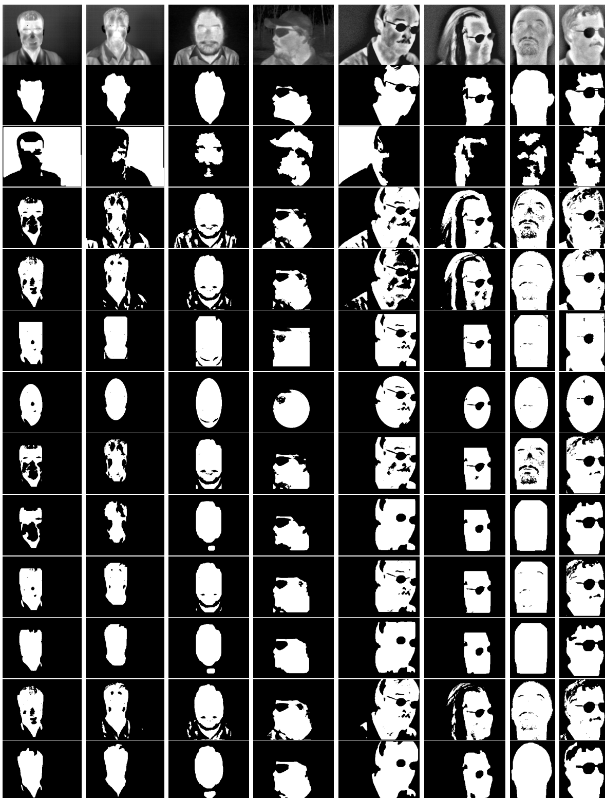
Fig. 10. Sample test set results for images from the UND database (columns 1 and 2), Terravic database (columns 3 and 4), IRIS database (columns 5 and 6) and FSU database (last two columns). Original images are in the first row and manual masks in the second. Approaches by [10], [11] and [12] are in rows 3 to 5 respectively. The remaining rows have the results of our proposals A to H , respectively.
