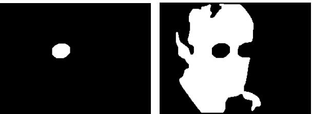
(e) Result of the morphological operator (opening) with a circular structuring sum element of 10 pixel radius. (f) Final result of the operation, after making the with a circular structuring sum.
