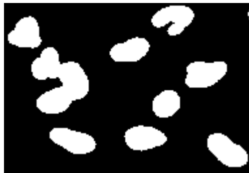
Figure 2.13: Result of Otsu's method applied to figure 2.9a.
