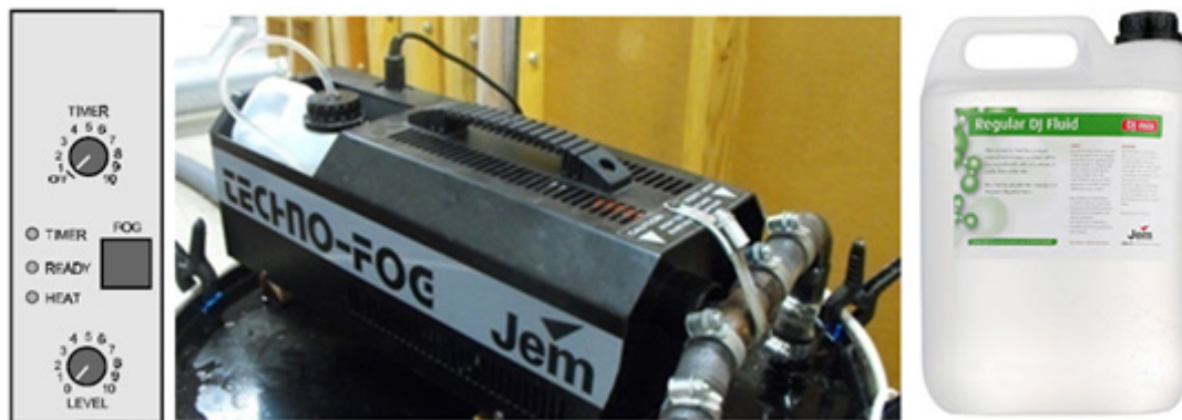
Figure 2.18. Smoke machine (middle), the remote control (left) and the seeding used for tracer (right).
