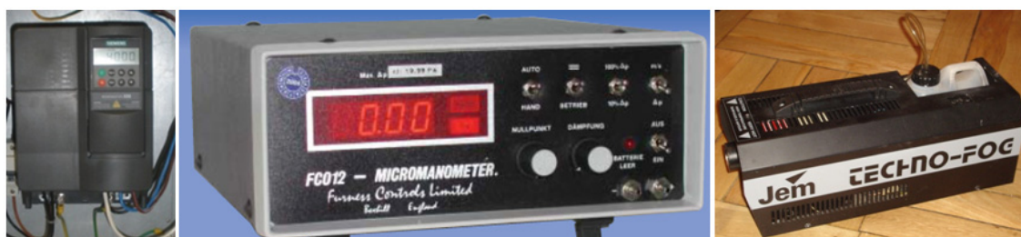
Figure 2.22. Left: electronic frequency converter device; middle: micromanometer; right: smoke machine.
