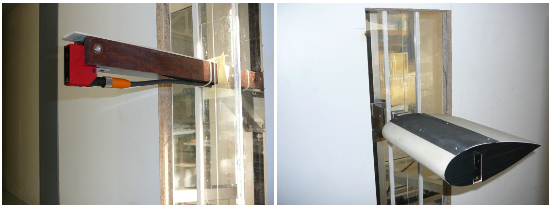
(a) Mast without the cowl, revealing the carbon-fiber inserts. (b) Mast with the cowl, made from a NACA0030 profile.
