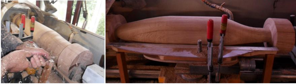
Figure 8-11 - Illustration of handwork during fuselage machining, and on the right, the intermediate shape of the fuselage.
