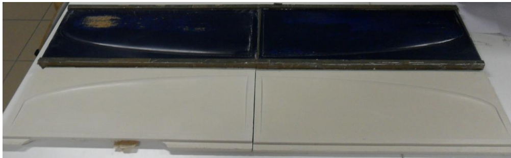
Figure 8-4 - Final plaster moulds.
