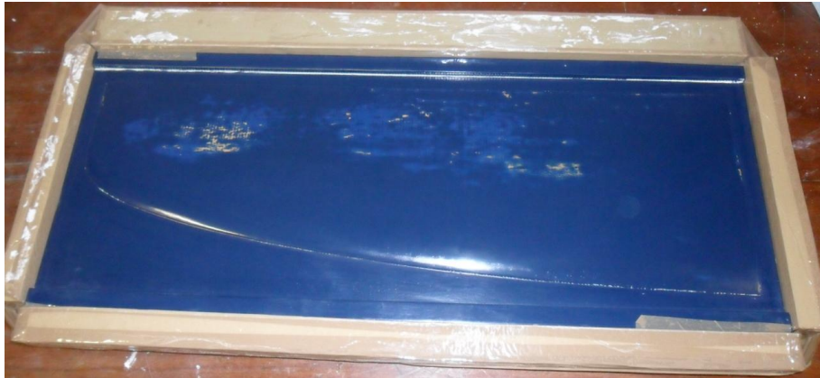
Figure 8-3 - Plug prepared to receive the plaster for mould construction.
