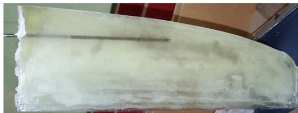
Figure 8-7 - Intermediate aspect of the wing. Corrections on trailing edge were applied to make it smooth and constant.
