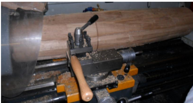
Figure 8-10 - Initial machining of the fuselage.
