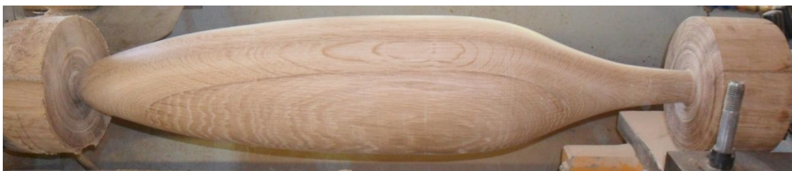
Figure 8-13 - Final machined shape of fuselage.
