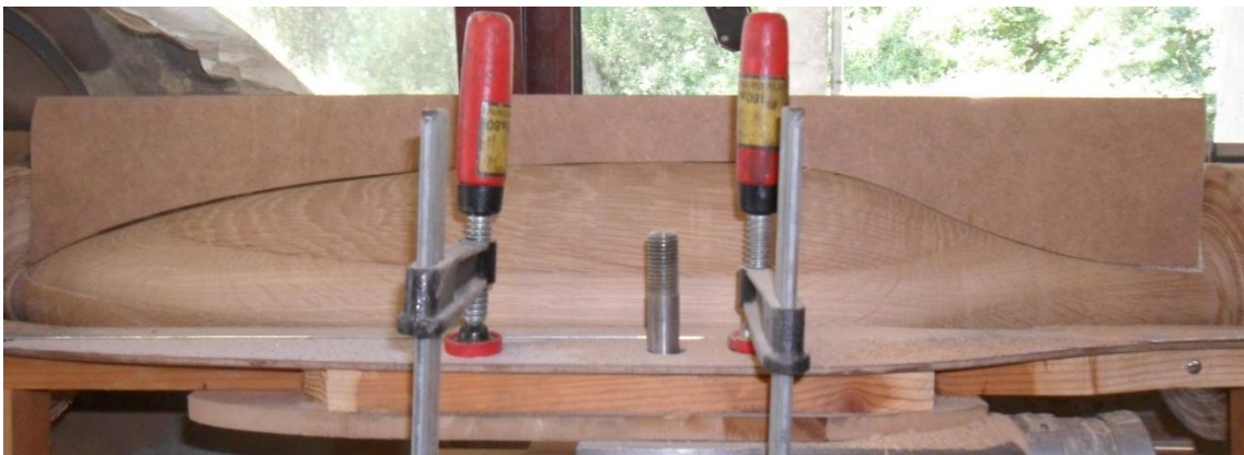
Figure 8-12 - Comparison between ideal shape and handwork machined shape. The small gaps present in this figure were eliminated later.
