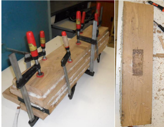
Figure 8-9 - Appearance of glued planks. On the image on the left is possible to watch all planks glued, and in the image on the right is showed the hole inside to accommodate extra ballast.
