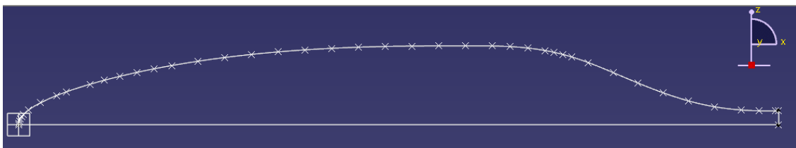
Figure 6-1 - Fuselage points in CATIA obtained from Excel.
