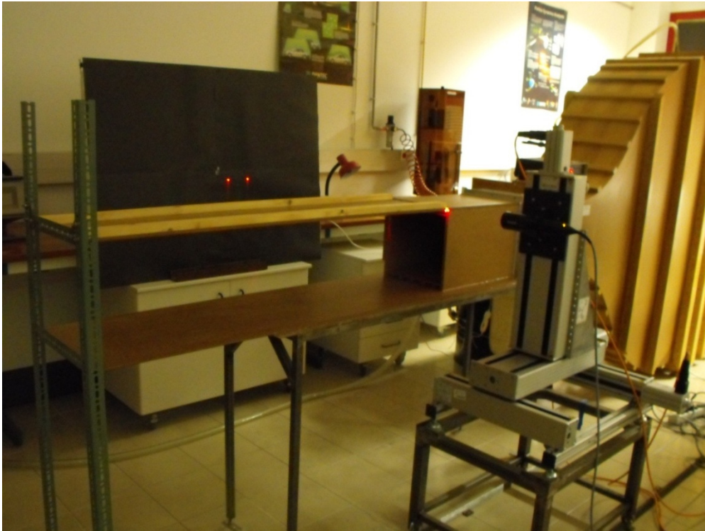
Fig. 8 Wind Tunnel and Test Section
