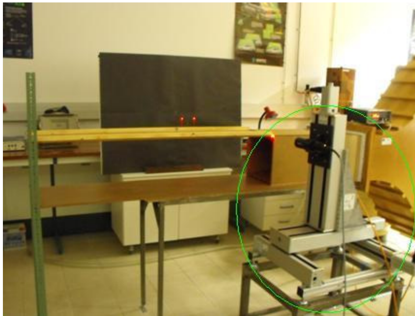
Fig. 13 Traverse System with the transmitting/receiving Optics System
