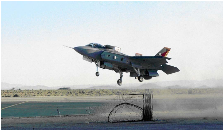
Figure 1.1 – Joint strike Fighter F-35B. V/STOL aircraft with an illustration of the ground vortex
