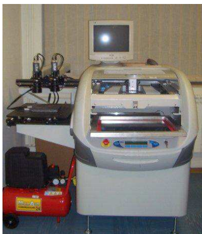
Figure 6.1 - DEK 248 printing machine
