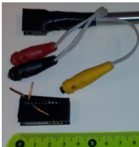
Figure 4.1.3.5 - Constructed adapters for try to resolve the background noise.
