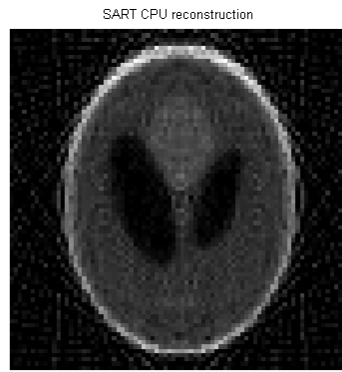
Figure 4.7: Shepp-Logan phantom ART reconstruction.
