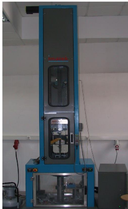
Figure 2.2 - Impact machine IMATEK-IM10.
