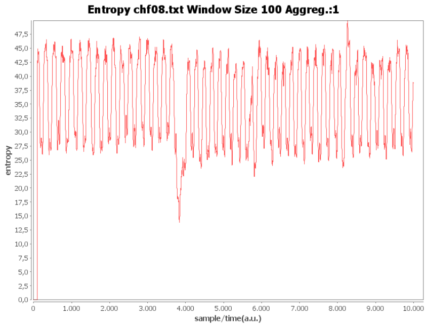
Figure 33. Evolution of entropy estimation in time for the chf08 non-healthy subject (mean value: 35.3840; standard deviation: 7.3688; amplitude: 26.1115), considering a moving window of 100 samples.
