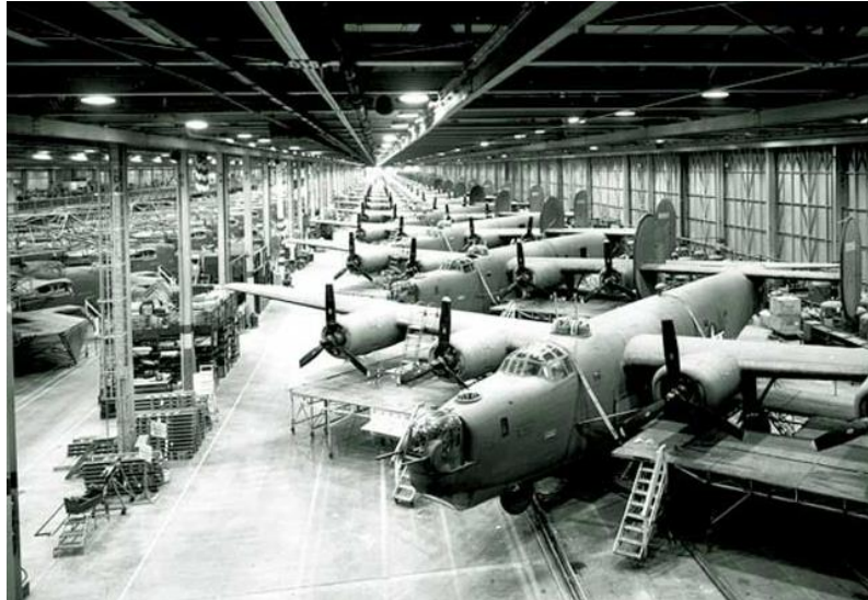
Figure 2.4 - Assembly line of the B-24. Note the rails to allow the movement of aircraft along the assembly line.
