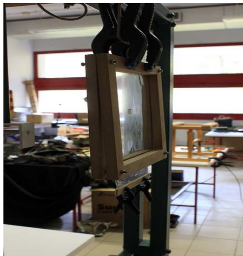
Figure 27 - Experimental setup to pre-tension the membrane [30].
