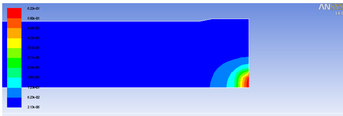
Figure 4.13: Contours of the Mach number near the throat for time \approx 5 s.
