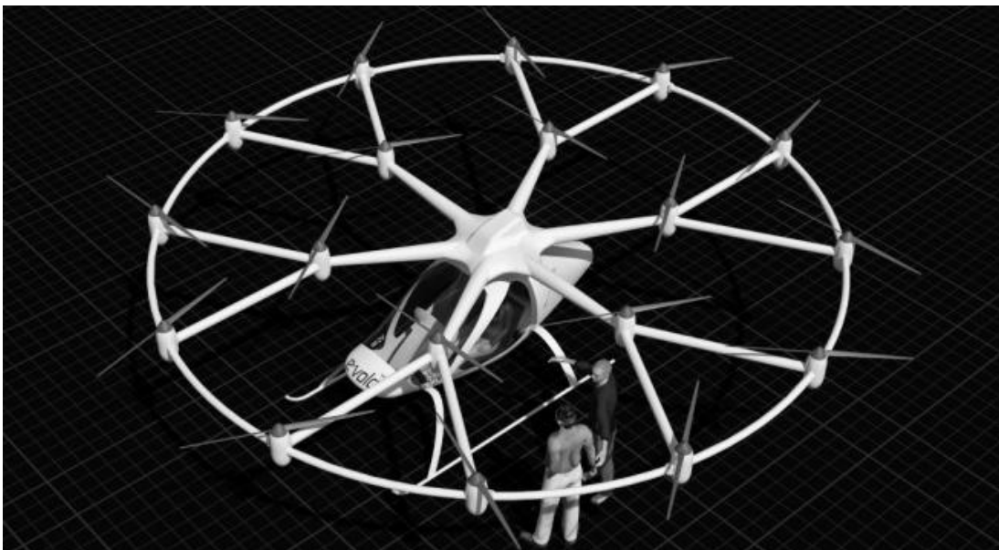
Figure 2.6 - Electric rotorcraft with 18 motors, VC200. [8]
