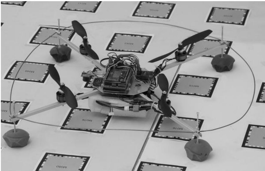
Figure 1.2 - Autonomous quadcopter that use a smartphone to navigate. [9]
