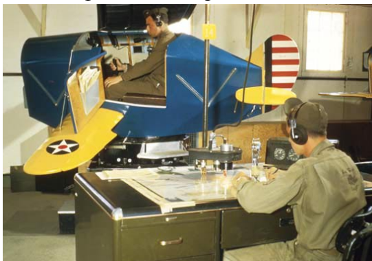
Imagem 06 – Simulador de voos militares, para fins de treino durante a Segunda Grande Guerra. Flight simulation in the C-3 Link Trainer, U.S. Army Air Forces, 1940s. A cadet takes the controls, and a nearby instructor relays commands by telephone.
