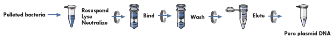
Figure 18: QIAprep Spin MiniPrep plasmid DNA purification procedure (adapted from QIAprep MiniPrep Handbook, 2006).
