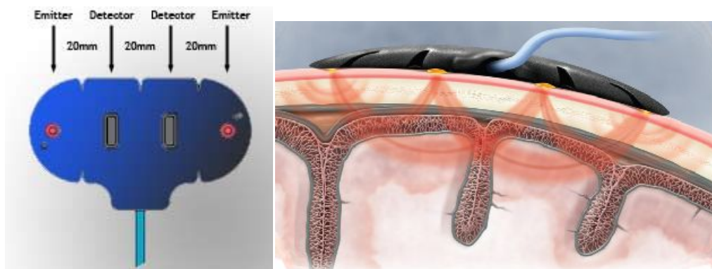
Figure 2. Image representing NIRS NONIN equanox technology.
