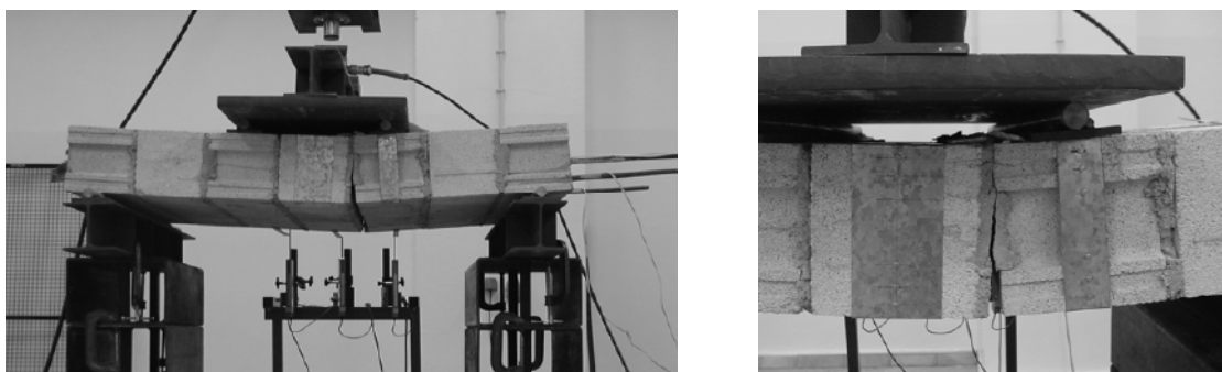
Figure 8 Typical wall failure
