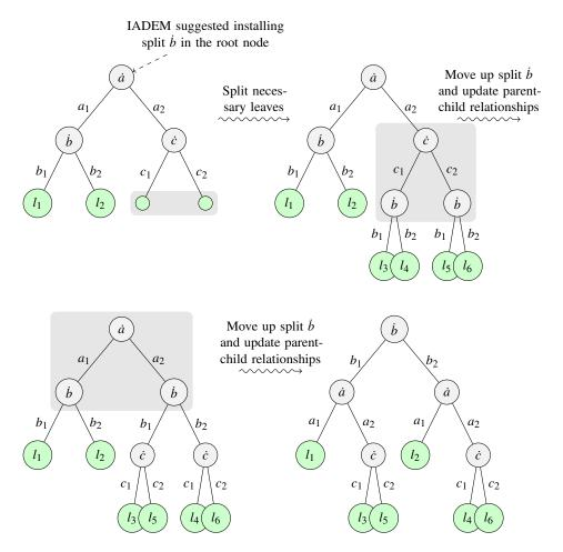
Figure 2. Algorithm 3 transforming a decision tree in order to install a different split (B) in the root node.
