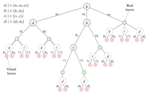
Figure 1. Example of a decision tree induced by the Online Hybrid Tree algorithm.
