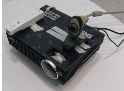
Figure 2. Projector-camera system used in AR X-Ray
