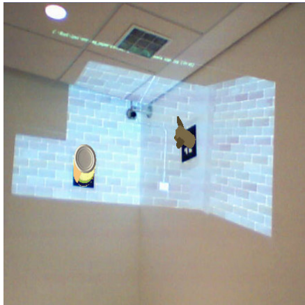
Figure 5. Successful ARTag registration with markers in front of projected light as seen by webcam
