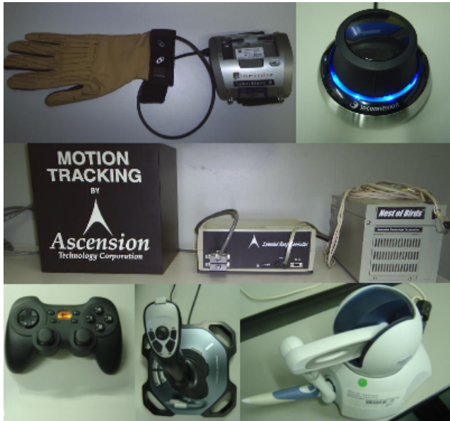
Figure 4. Example of devices supported by the EnCIMA engine (left to right, top to bottom): data glove, 3D mouse, 3D tracker, wireless joypad, force feedback joystick, and phantom haptic device.
