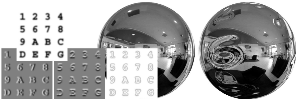
Figure 9. A bump map (upper left) is converted to a normal map (lower left: separated RGB channels), which is used to deflect the per-pixel normal from its original direction (mid) to let a relief appear on the surface (right).
