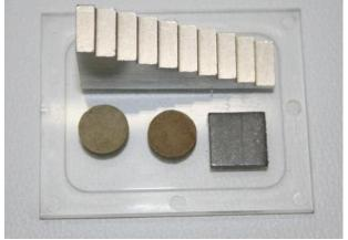
Figure 1: Specimens, aluminum step wedge and lead plate.
