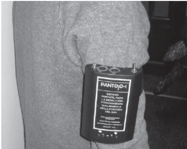
FIGURE 4 – Arm circuit of the gaze tracker. The EOG signal processing is located in this box, as well as the wireless circuitry to communicate the gaze position to the mouse driver installed in the Computer.
