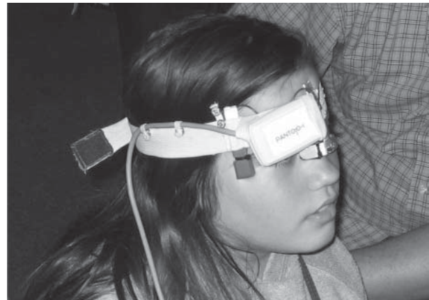
FIGURE 3 – Head-band of the gaze tracker. Note the amplifier circuit is located only a few centimetres away from the electrodes. The central electrode is applied on the nasal septum and the two lateral electrodes on the temples. The cable conveys the pre processed EOG to an arm circuit with a wireless link to a computer.
