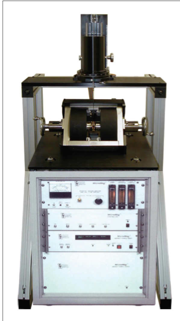
Figure 2.1: The Princeton Measurements Corp. Model 3900 MicroMag™ Vibrating Sample Magnetometer (VSM)
