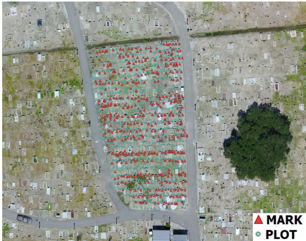
Figure 17. Raw data captured using RTK equipment, overlaid onto UAS generated orthomosaic. Blue dots represent the corners of each burial plot, and red triangles represent the location of burial markers.
