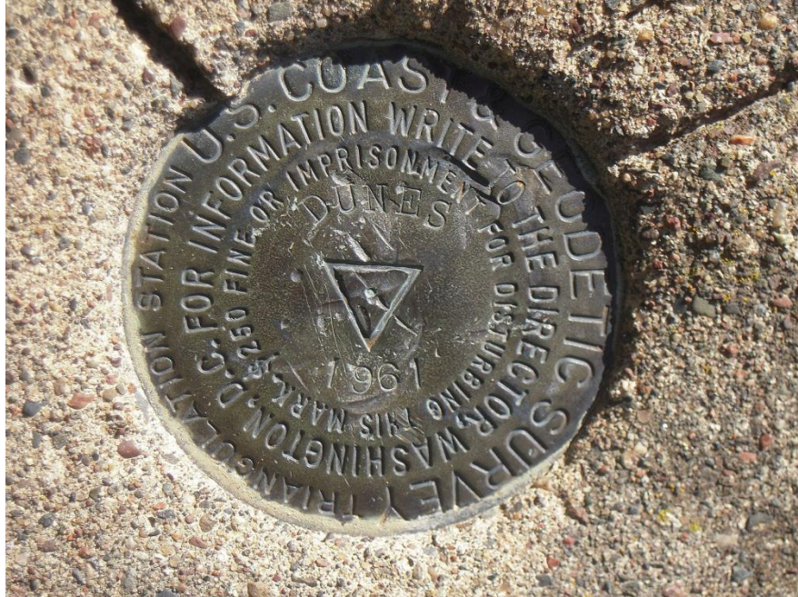
Figure 16. This image represents the typical marker used for NGS survey points. These markers are fixed into the ground and are intended to be immovable. ( https://commons.wikimedia.org/wiki/File:United_States_National_Geodetic_Survey_marker_QO1858.jpg )
