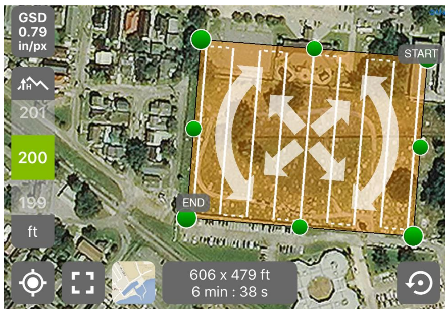
Figure 18. This screenshot was captured from the smart phone used to pilot the Unmanned Aerial System. The application used, Pix4d Capture, allows users to select a survey area and an altitude and then automatically generates a flight plan and triggers the UAS camera at the appropriate time in order to generate accurate spatial data.
