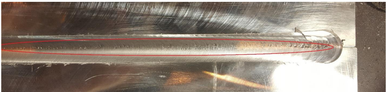
Figure 4.7: Lack of Consolidation Welds 3 & 6
