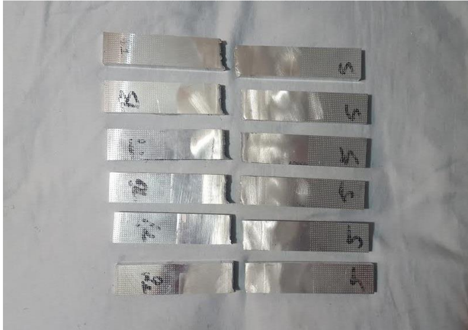
Figure 4.5: Weld #5 Post Tensile Break
