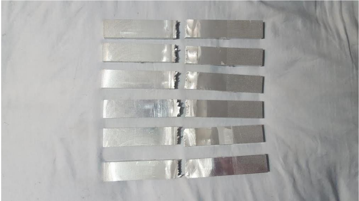
Figure 4.6: Weld #6 Post Tensile Break
