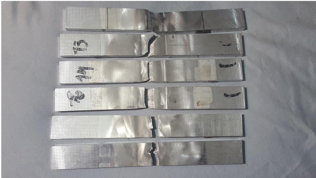
Figure 4.1: Weld #1 Post Tensile Break
