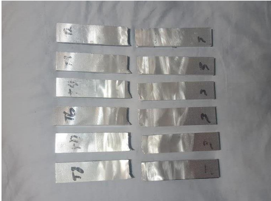
Figure 4.3: Weld #3 Post Tensile Break
