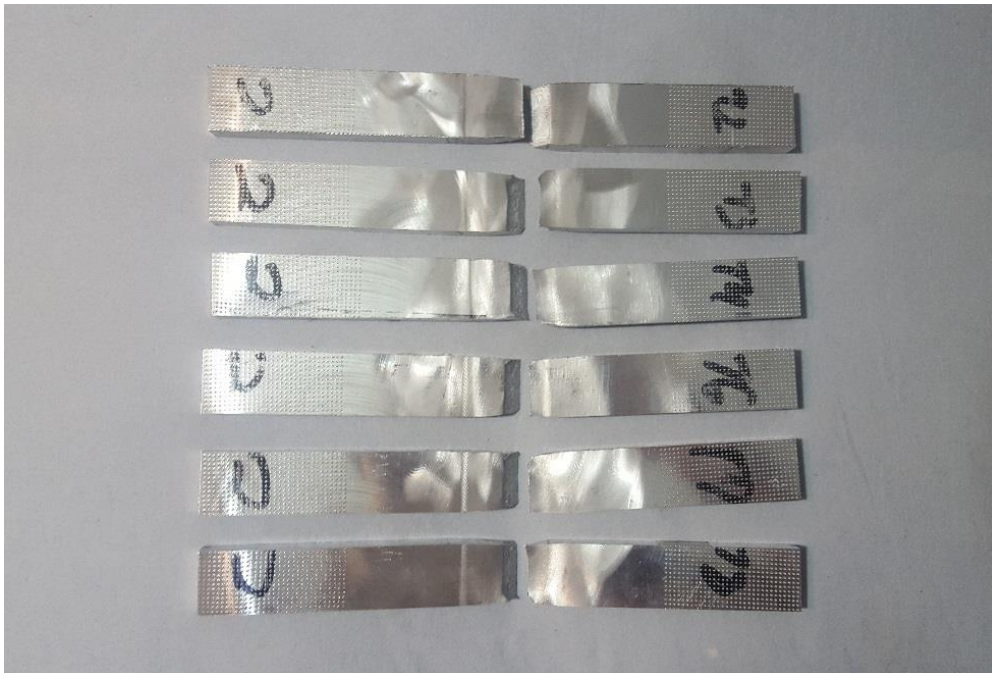
Figure 4.2: Weld #2 Post Tensile Break
