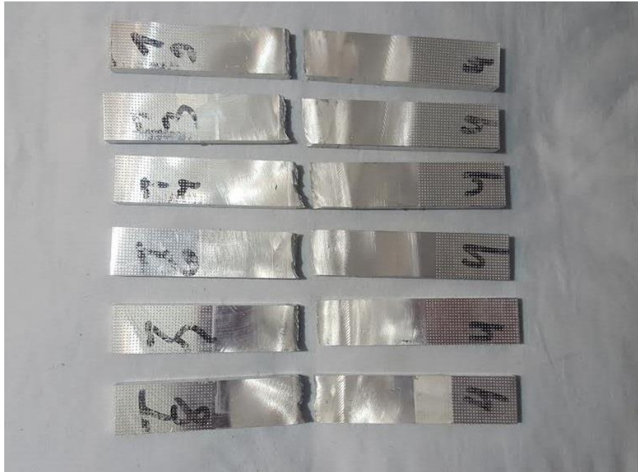
Figure 4.4: Weld #4 Post Tensile Break
