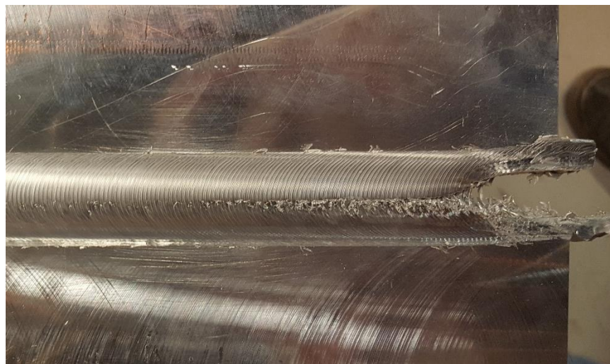
Figure 4.9: Lack of Consolidation
