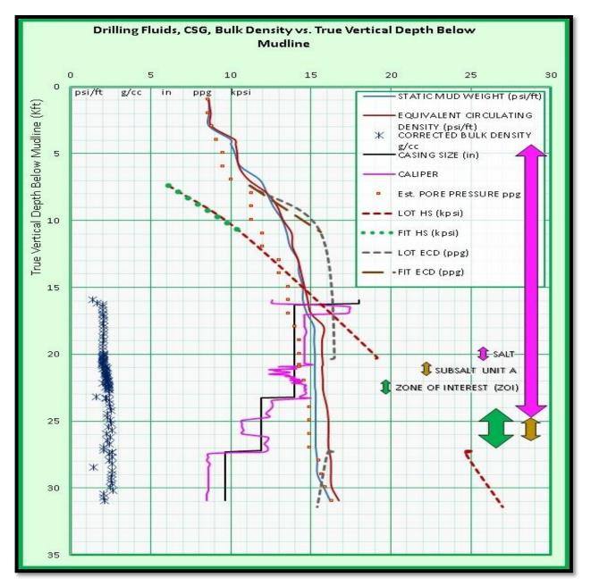
Graph 9. Composite graph showing drilling fluid pressure gradients, Casing and bit size comparison, Corrected bulk density, Formation integrity and Leak off tests. Salt, Zone of Interest, and Subsalt unit A represented by the Pink, Green, and, Brown arrows (respectively). Graph created using BSEE well log data and MS Excel 2013.
