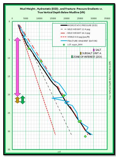
Graph 7. Mud weight, Annular PWD ECD, and fracture pressure gradient, versus true vertical depth below mudline (kft). Pink, green, and brown arrows indicate Salt, ZOI, and Subsalt Unit A (respectively). Graph created using MS Excel 2013.
