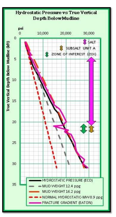
Graph 1. Graph showing mud weight and hydrostatic information. Hydrostatic equivalent circulating density while drilling or (annular PWD ECD) is the thick black dataset. Mud weight (16.2 ppg) is red dash/dot dataset. Normal hydrostatic is red dashed dataset, and fracture gradient is in pink solid dataset. Note the downscale deflection in fracture gradient when passing through Base of Salt at approximately 21,000 ft. Graph created using MS Excel 2013.
