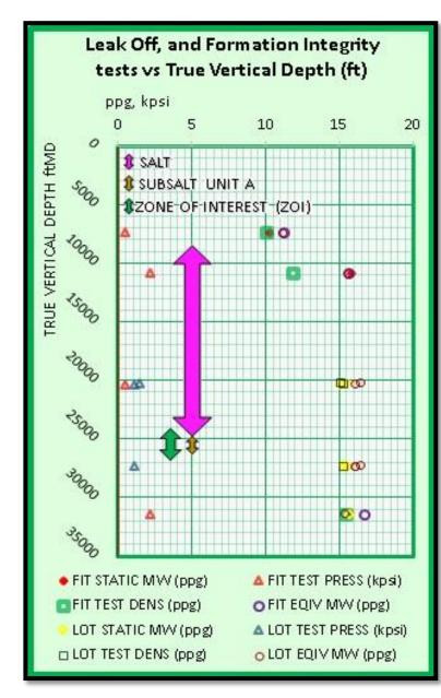
Graph 8. Leak off Test and Fracture Integrity Test graph. Data compiled from mud-log report. Graph created using MS Excel 2013.
